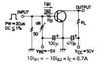
(For PNP, the polarity is reversed.) Unit (resistance :  $\Omega$ , capacitacne : F)
